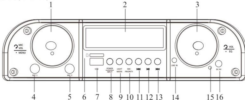
1. MIC Volume/Menu: Rotate the dial to adjust microphone volume. Push the dial to enter the menu and adjust microphone bass (1b) and treble (1t).
